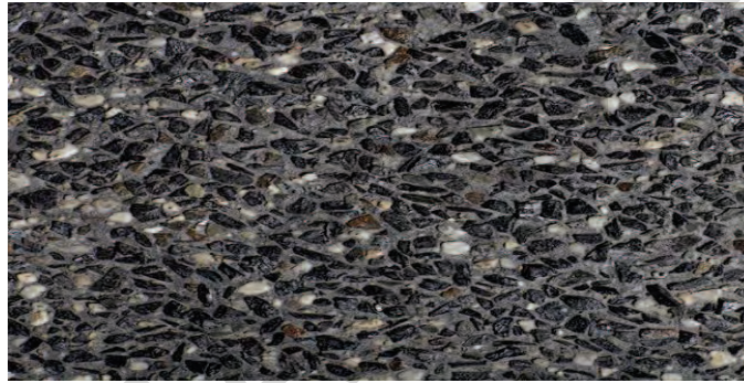
Example of exposed aggregate concrete.
