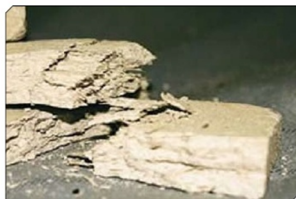
Figure 19: These pieces of broken asbestos cement sheet are not fixed or installed.
