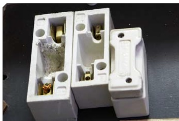
Figure 17: Friable asbestos insulation in an electrical fuse housing.
