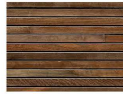
T2 - FEATURE TIMBER FACADE CLADDING & FRONT ENTRY DOOR TO HAVE NATURAL TIMBER STAIN FINISH
